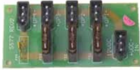
S577 – Power Distribution
