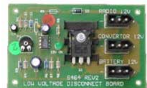
S464 – Low Voltage Disconnect Board
